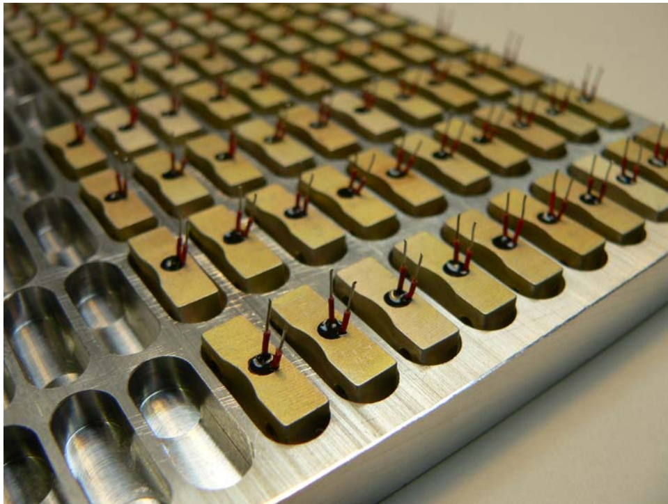
Sensors being epoxied into small cold plates
